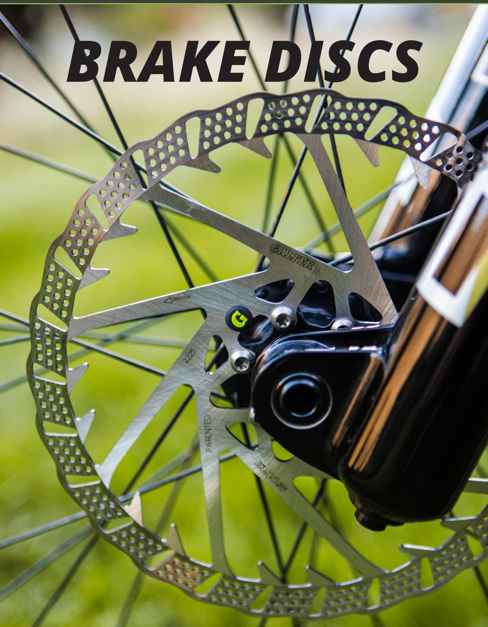
UK Laser-cut from high-carbon stainless steel, they are a direct application of top-competition technology made available to all users. They replace the original discs without the need for adaptation or manipulation. Made in Spain, all Galfer brake discs have anti-corrosion treatment, are lighter than most discs on the market and do not emit noise or vibration.
